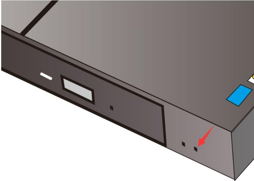
Press button in this hole with a needle and hold more than 2 seconds then release, CDRip will be reset.
